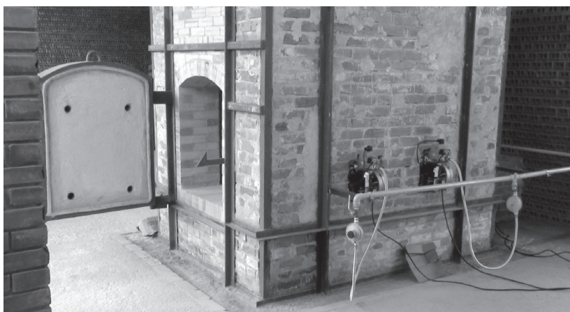
FIGURE 2 - Gas kiln set up in the Cabo Handicraft Center
